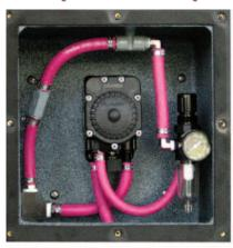
Knight's FoamClean Mobile and Wall Mount system is powered by 5 GPM (18.9 LPM) Polypropylene double-diaphragm pump with Viton or Santoprene seals or 4 GPM (15 LPM) pump with Teflon seals for extended product life, giving you maintenance-free pump operation. The pump is protected in a chemical and corrosion resistant Polyethylene case protecting the pump for years of reliable service.
