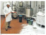
The dryness or wetness of the foam can be adjusted for different cleaning applications with a simple turn of a knob.
